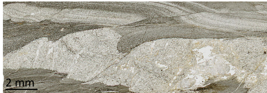
Boudinage of sandstones
