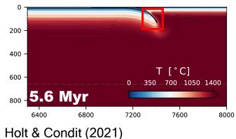
Spontaneous, buoyancy driven subduction model (Holt & Condit, 2021), using ASPECT\*
