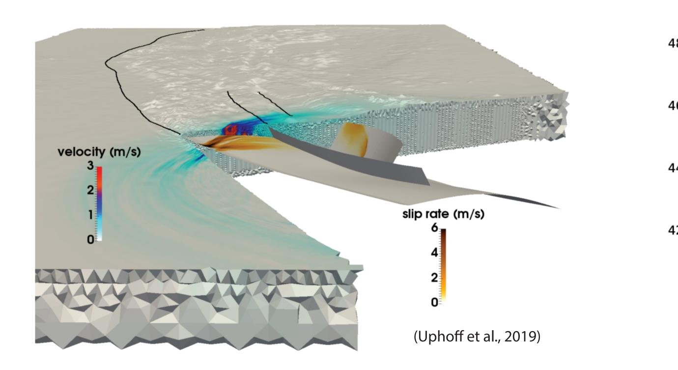
Dynamic rupture simulation of a subduction zone megathrust rupture, including activation of seaward and landward verging splay faults. Colors show slip rate on the faults and particle velocity (shaking) in the solid.
