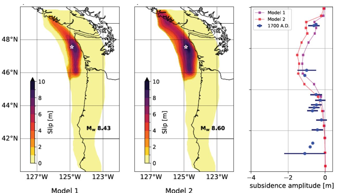
Dynamic rupture simulations for Cascadia, exploring different scenarios and comparing with coastal subsidence measurements from the 1700 event (right).
